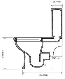
DIAGRAMS NOTTO SCALE | ALL DIMENSIONS IN MM TOLERANCE OF  $\pm$  5MM  ${\it ALL PRODUCTS CONFORM TO BRITISH STANDARDS }$
