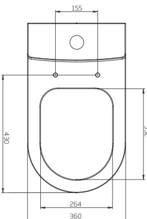
DIAGRAMS NOT TO SCALE | ALL DIMENSIONS IN MM TOLERANCE OF  $\pm 5\text{MM}$
