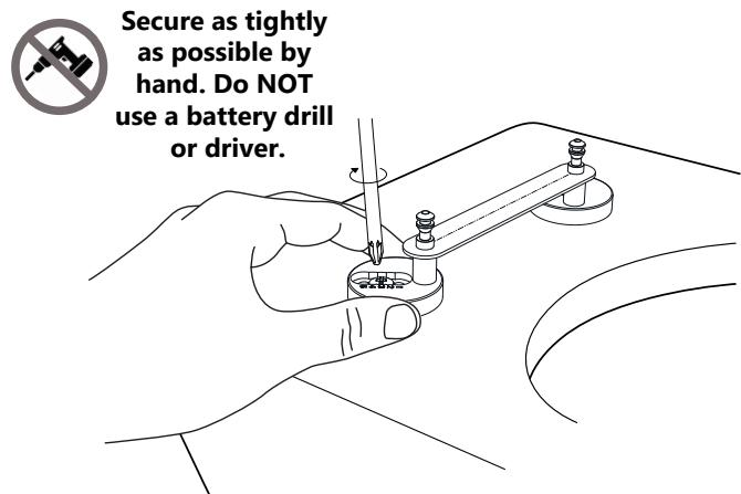
4 Remeasure the distance, making sure the 438mm dimension is met and remove the template and add the cover cap.
