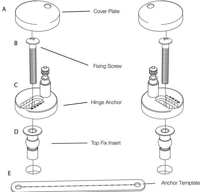
Note - alternative nuts and washers are supplied if you wish to secure the seat from underneath the deck of the toilet pan. If so dispose of the black top fix inserts and tighten with the securing key supplied.
