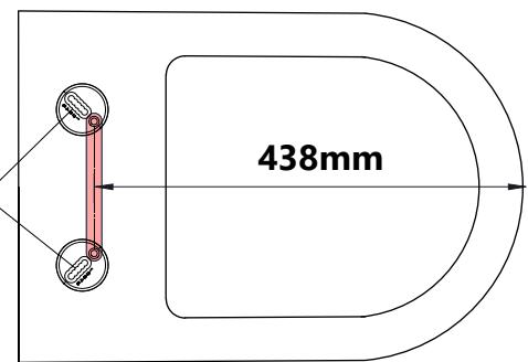
3 Once the 438mm dimension shown above is met and the template is parallel to the back edge, insert the bolts then tighten using a screw driver.
