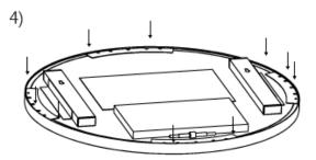
5) Connect the LEDs to the electronics box via the connector cable and secure the connector to the back of the mirror using the clips on the back of the mirror.
