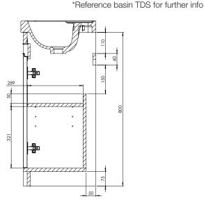
Diagrams not to scale All dimensions in mm Tolerance of +/-5mm Handle included in diagram
