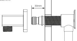
Once final surface is in place, assemble the wall elbow and secure with grub screw.
