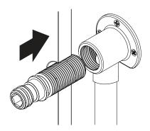
For square elbows, ensure there is 30 mm (±1mm) of the fixing thread in front of finished surface to allow wall elbow to be attached securely. Round elbows have an adjustable plate, which gives a tolerance of ±5mm.
