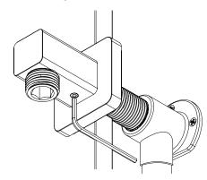
NOTE: If the wall elbow is positioned in an area subject to frequent and heavy mositure, it may be required to seal the outer edge of the elbow with silicone.
