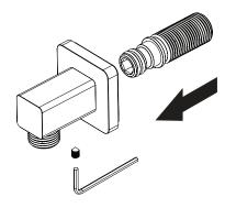
Connect fixing thread to plumbing fitting. (Diagram shows use of plumbing elbow - not supplied)
