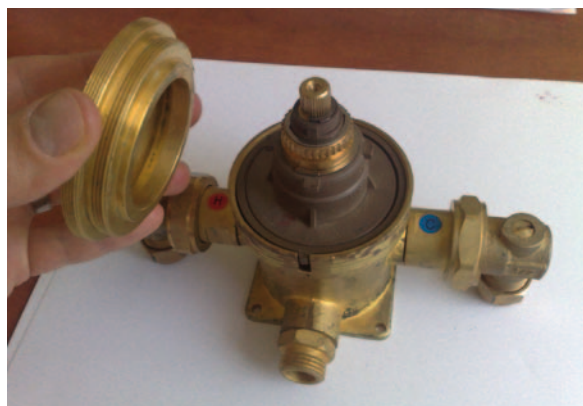
1.8 Remove the flow control stop ring remembering the original position for later re-installation.
