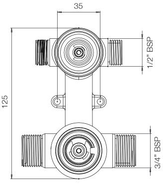
NOTE: VALVE TO BE RECESSED 80-100mm FROM FINISHED WALL SURFACE
