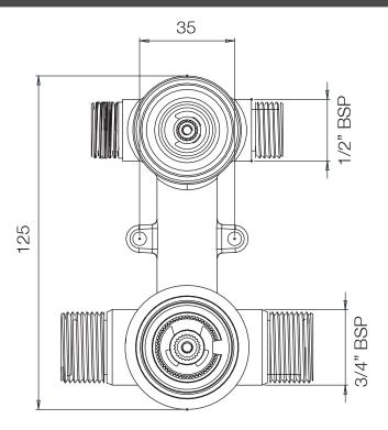
NOTE: VALVE TO BE RECESSED 80-100mm FROM FINISHED WALL SURFACE
