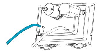
5. Make sure the cistern is fully commissioned before mounting the bracket in place.
