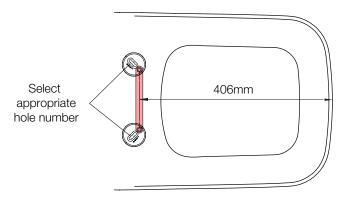
3 Once the 406mm dimension shown above is met and the template is parallel to the back edge, insert the bolts then tighten using a screw driver.
