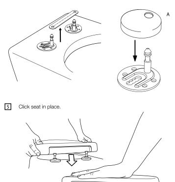
If difficult to push in, lubricate the rubber insert with water.
