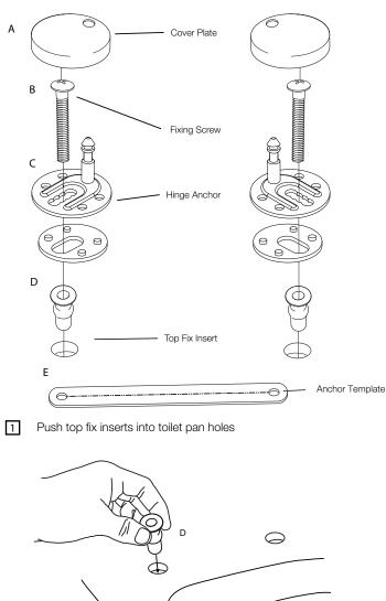
2 Place the template over the anchor pins, selecting the appropriate hole numbers (on the anchors) so that the 406mm dimension from the front of the pan to the centre line of the template is met.
