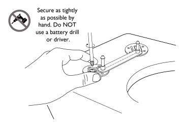
4Remeasure the distance, making sure the 406mm dimension is met<br/>and remove the template and add the cover cap.
