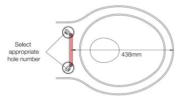
3 Once the 438mm dimension shown above is met and the template is parallel to the back edge, insert the bolts then tighten using a screw driver.
