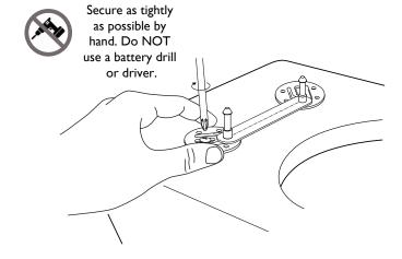
Remeasure the distance, making sure the 438mm dimension is met and remove the template and add the cover cap.
