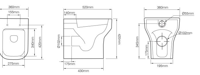
\*Dimensions are subject to change, customers are advised to measure actual product before commencing installation. \*\*Fixing point dimensions are for guidance only. The positions of fixings must be checked when product is received.
