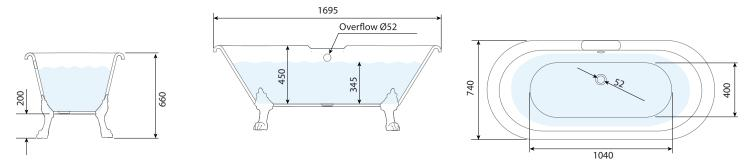
\*Dimensions are subject to change, customers are advised to measure actual product before commencing installation. \*\*Fixing point dimensions are for guidance only. The positions of fixings must be checked when product is received.
