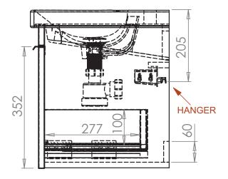
Diagrams not to scale All dimensins in mm tolerance of +/-5mm
