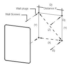
To secure the mirror further, a small amount of silicone sealant can be applied to the side of the extrusions to prevent the mirror being accidently pulled away from the wall. To remove the mirror, the mirror should first be lifted and then pulled away from the wall.
