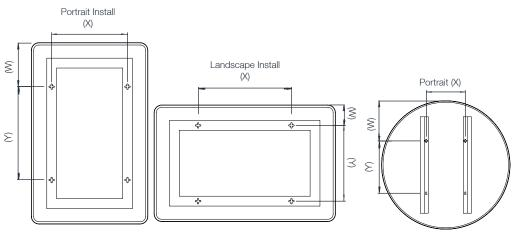
3) On your mirror, measure the distance (W) between the top of the mirror and the top keyhole slot. From position A (marked in the previous step) measure vertically down distance (W) and mark with a pencil. This is position B.
