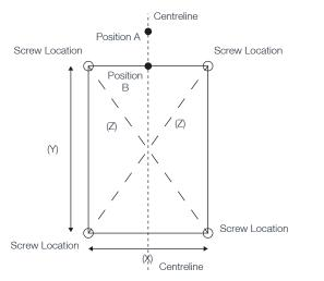
1) On the wall, using a spirit level and pencil, draw a vertical line to represent the position of the centreline of the mirror.
