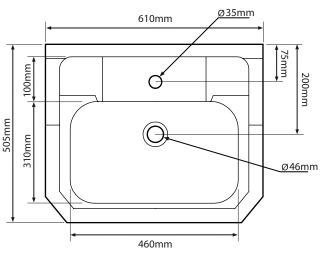
DIAGRAMS NOT TO SCALE | ALL DIMENSIONS IN MM TOLERANCE OF  $\pm$  5MM  ${\it ALL PRODUCTS CONFORM TO BRITISH STANDARDS }$
