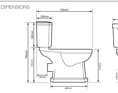
DIAGRAMS NOT TO SCALE | ALL DIMENSIONS IN MM TOLERANCE OF  $\pm$  5MM \$ ALL PRODUCTS CONFORM TO BRITISH STANDARDS \$
