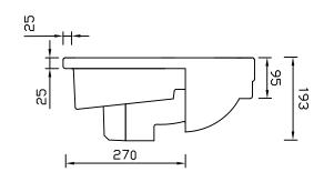
\*Dimensions are subject to change, customers are advised to measure actual product before commencing installation. \*\*Fixing point dimensions are for guidance only. The positions of fixings must be checked when product is received.
