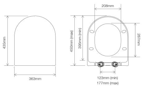
\*Dimensions are subject to change, customers are advised to measure actual product before commencing installation. \*\*Fixing point dimensions are for guidance only. The positions of fixings must be checked when product is received.
